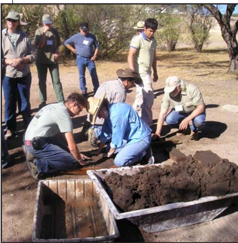
Left: Participants get their hands dirty making adobe bricks. Right: Boiling alum, which is then applied to adobe bricks as a traditional waterproofing technique.
